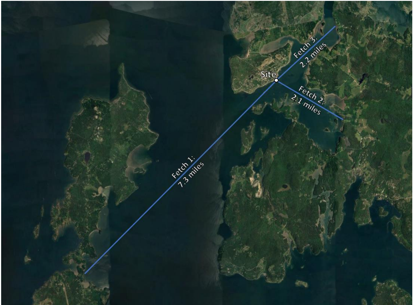
Attachment 9 Figure 5: Fetch Lines Used in Fetch Limited Wave Calculations
