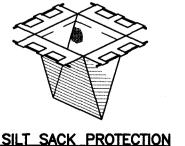
PRIOR TO FINAL GRADING AND PAVING OPERATIONS BEGIN, A CATCH BASIN INSERT (SUCH AS A SILT SACK OR A DANDY BAG II) MUST BE INSTALLED IN EACH BASIN PER MANUFACTURES INSTRUCTIONS. HAY BALES SHOULD BE REMOVED ONCE INSERTS ARE INSTALLED.
