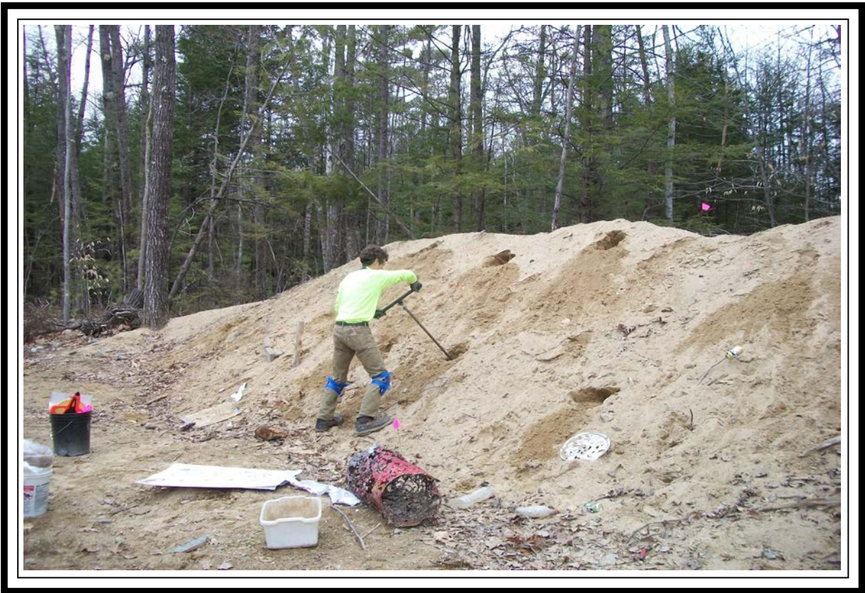
Collecting a soil sub-sample from the front berm face of the pistol range
