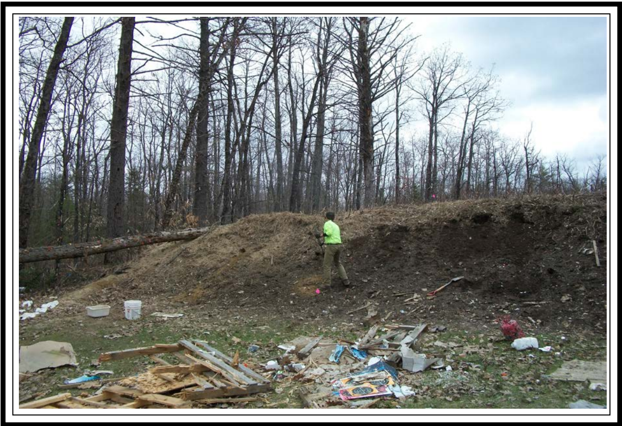
A soil sub-sample being collected from the front face of the rifle range berm
