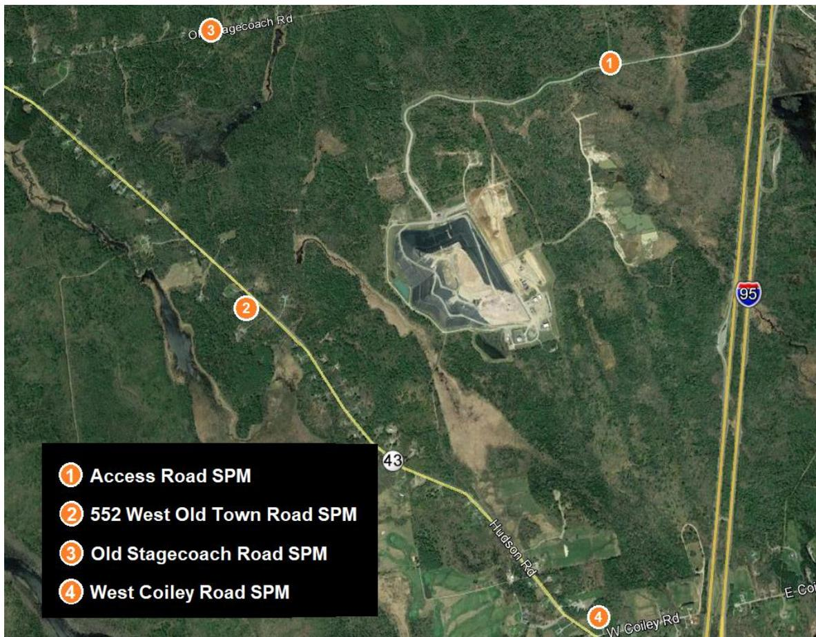
Figure 1-1 Juniper Ridge Landfill  $H_2S$  Single Point Monitoring Locations
