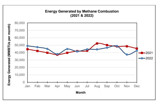
Figure 5-1 Energy Generated by CH4 Combustion at the JRL Flare, 2021 & 2022
