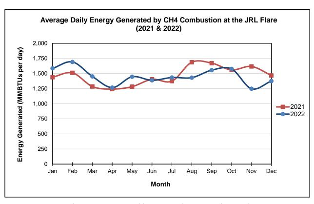
Figure 5-2 Avg. Daily Energy Generated by CH<sub>4</sub> Combustion at the JRL Flare, 2021 & 2022
