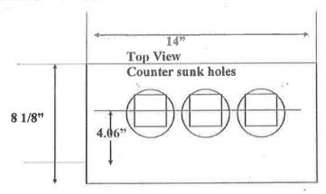
Size; 1" x 14" x 8 1/8" Blade Double Bevel Flat Bolt Size = 3/4" x 2 3/4"
