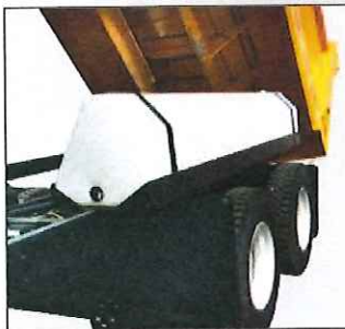
Optional pre-wet liquid tanks* installed inside fenders for protection.
