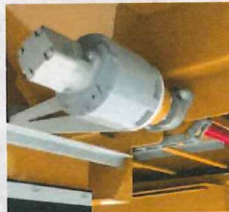
Main conveyor is driven through planetary drive mechanism utilizing a 10 cu in displacement motor and 2" diameter driveshaft.
