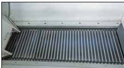
30.25" wide conveyor with 1/2" bars and dual 6:1 gearbox drive (standard on chain bodys)
