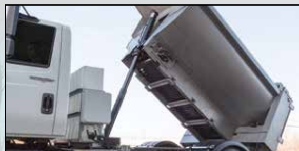
Multi-stage, double-acting, nitrided cylinder, trunnion-mounted hoist
