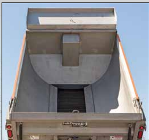
Unique, roll-formed sides and cross member-less design
