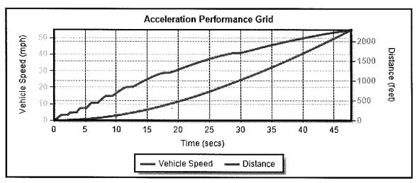
Acceleration Performance: TIME TO ACCELERATE ON A GRADE TO 55.0 (MPH) IS 47.84 (SECS)
