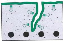
Step 2. Apply DECK-SIL® EP 1700 treatment to heal and seal surface.
