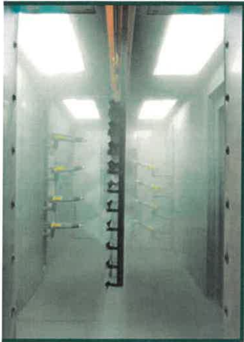
Electrostatically charged powder adheres to the RIB-BAK U-channel posts.
