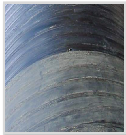
Step 4: Visually inspect the joint to ensure that male and female threads are engaged.
