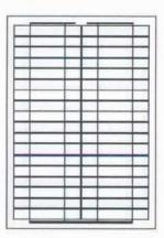
Laminate: Glass /EVA / TPT (tedlar/pet/tedlar) or TPE Front Side: High-transmission 3.2mm tempered glass Back Side: TPT /TPE Frame: Clear anodized aluminum frame Output: Junction box
