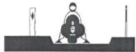
a) Single Stake used to augment an existing fixed object such as a fence post. Note the use of a blazer to provide a second reference point.
