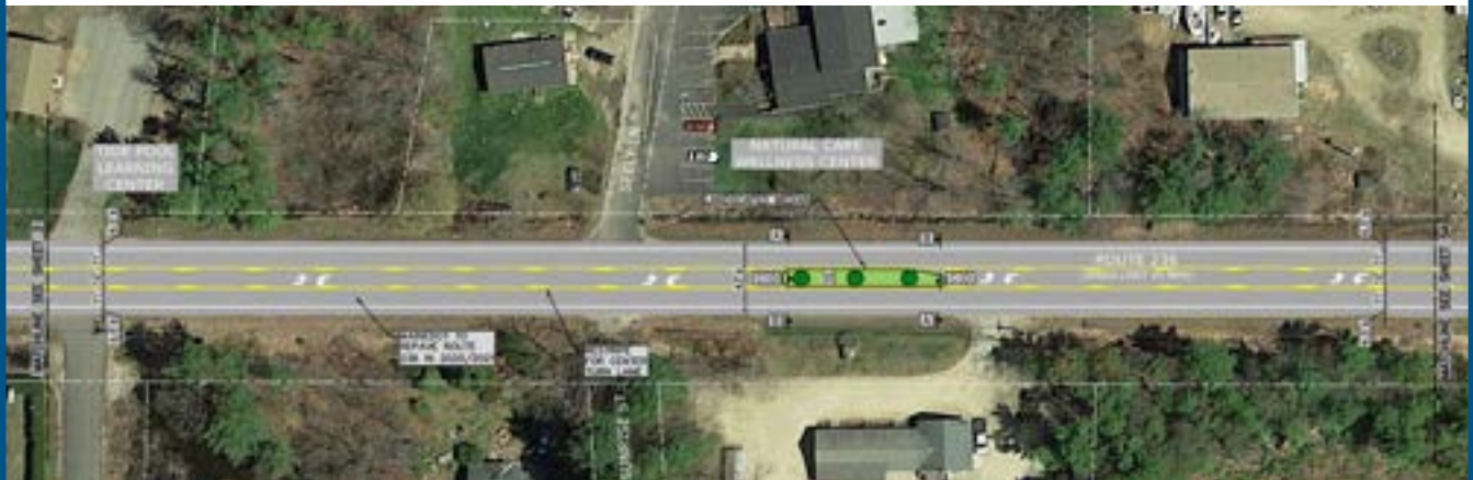
A concept from the Route 236 Corridor Study (2019) showing a center turn lane and planted median on Route 236 northwest of Bolt Hill Rd.
