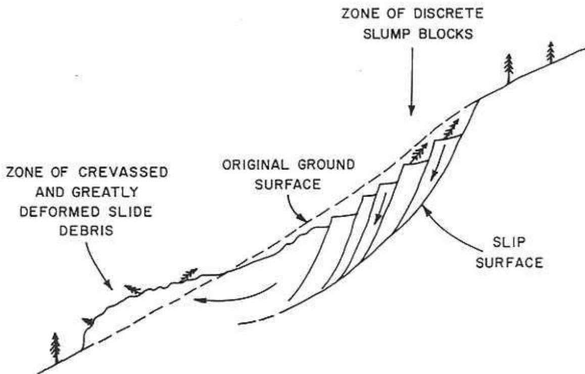
**Figure 1.** Cross section of a slump (from *W. B. Thompson, 1979, Surficial Geology Handbook for Coastal Maine: Maine Geological Survey, following p. 36*).
