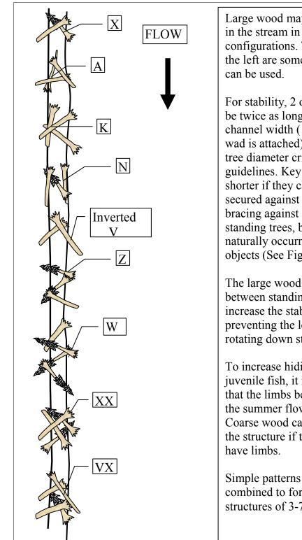
Figure 4. Showing typical plan view wood configurations and alphabet codes for use in describing them.
