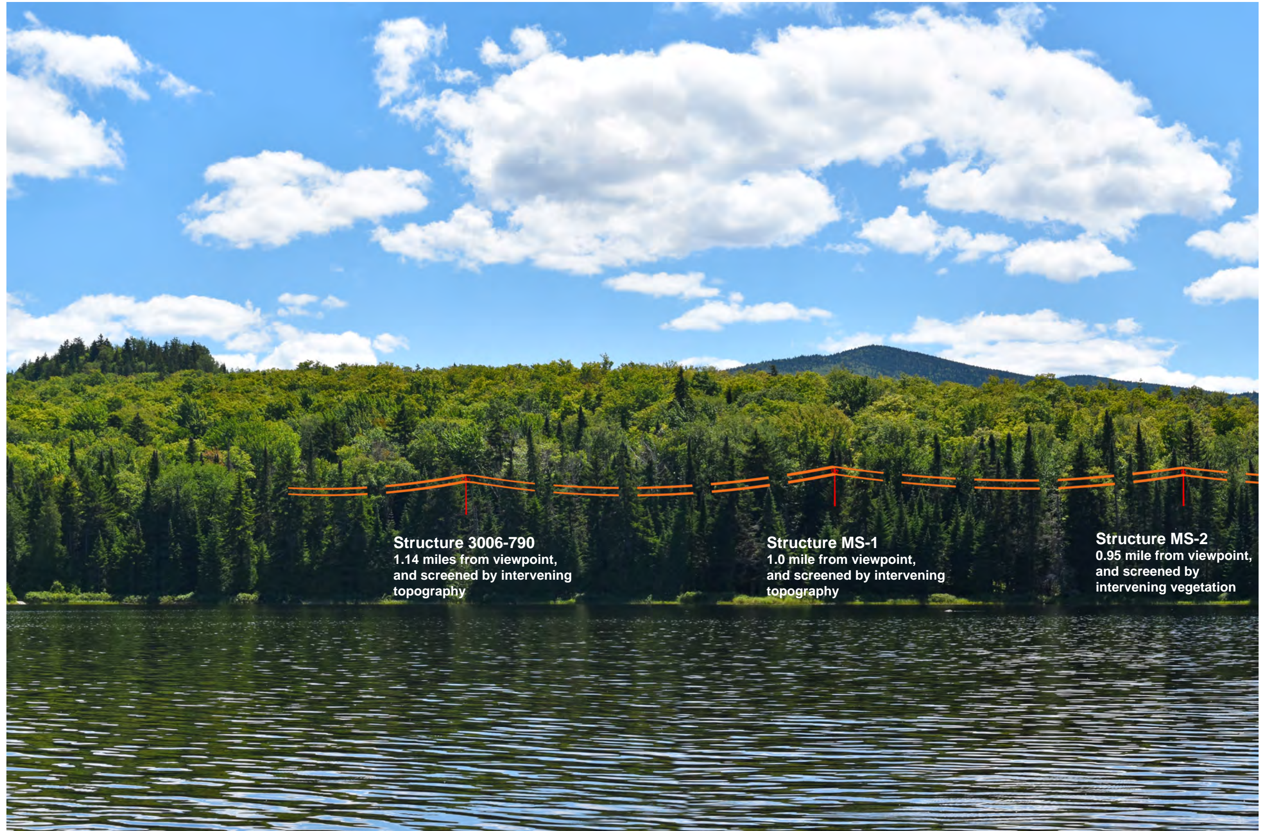
3D Model Illustration: Normal view looking southeast from the northern end of Beattie Pond toward the proposed Merrill Strip Twp Alternative of the HVDC transmission line. Based on the Alternative route, no structures, conductors, or shield wires would be visible from the Pond looking in this direction due to intervening topography and/or vegetation.
