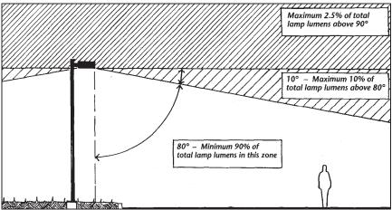
Figure 10.25,F-1. Cut-off fixture as defined by IESNA.
