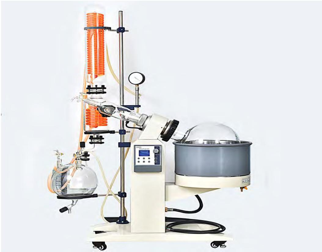
Rotary Evaporator (Roto Vape) – Used in Marijuana Distillate Production
