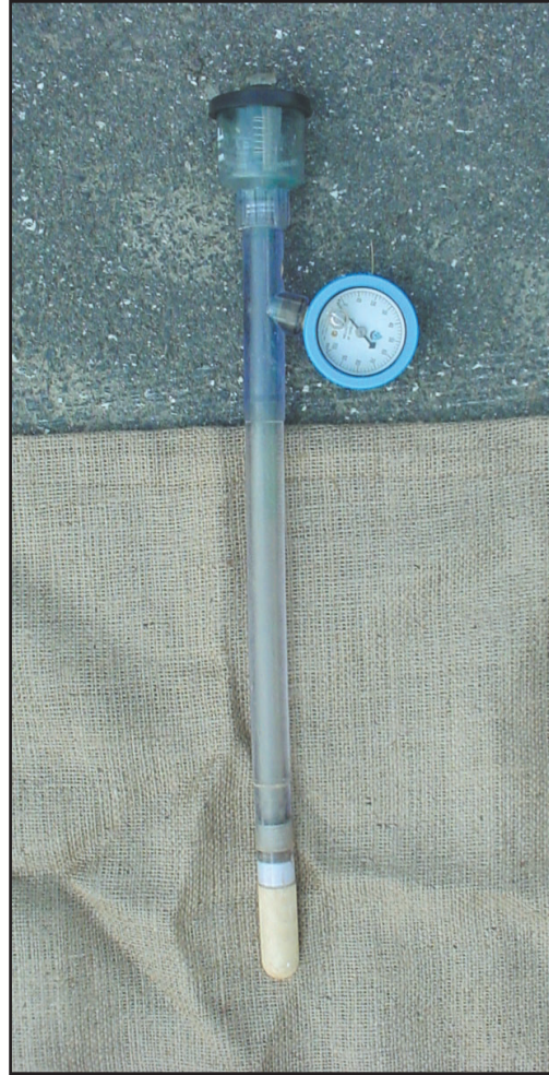
Tensiometer measures soil tension.
