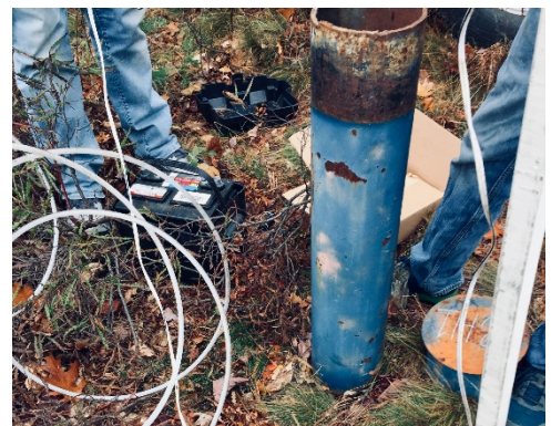
Figure 2. Well head at the Deblois 2 site with sounding tape, HDPE tubing, post-sample extraction and pre-decontamination.
