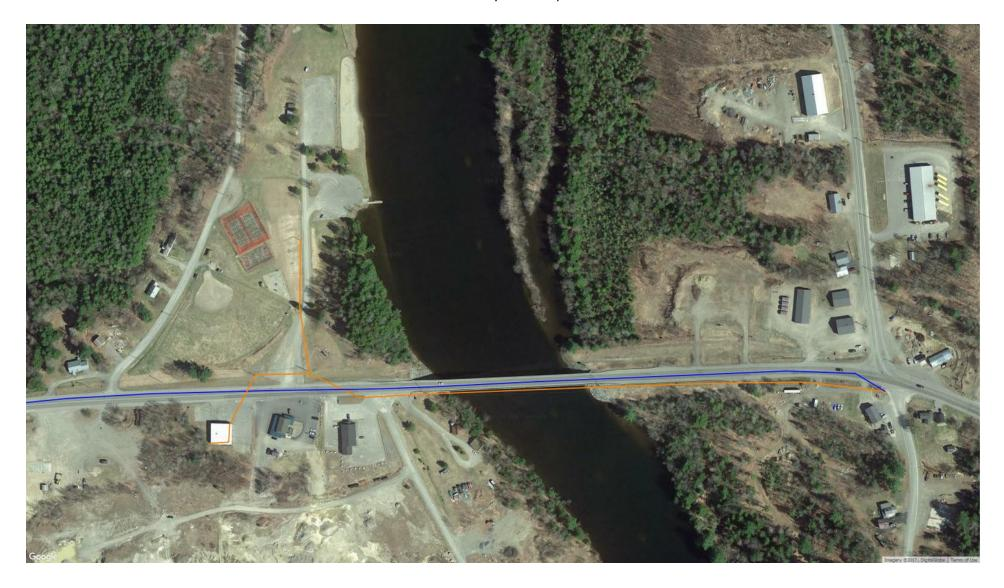
In the above image, the orange line represents new fiber construction while the blue line represents an existing 3RB fiber which will be used to transport broadband service from Millinocket to Medway. This plan is to provide service to the hotspot project outlined in Appendix A-1 and the currently vacant Nissen Building.
