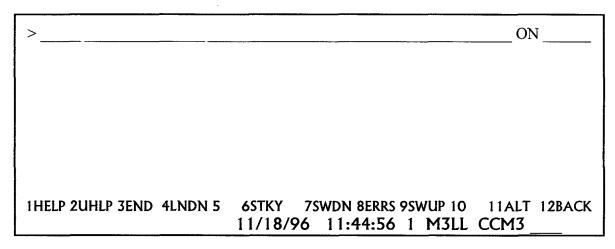
The only exception to this is the addition of PF11. Millennium 3.0 can potentially have up to thirty-six (36) function keys. Since only twelve (12) function keys can be displayed at the bottom of a screen, three sets of function keys can be defined and displayed in succession by pressing PF11. The MFASIS Technical Team has defined all three sets of function keys exactly the same. Therefore, pressing PF11 will always display the same set of function keys. The current function keys are as follows:
