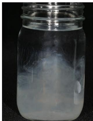
*In these photos, the bottles on the left contain distilled water with no minerals (zero hardness) while the bottles on the right contain minerals. The bottles on the right turn cloudy after adding a product that mimics glyphosate while the bottles on the left remain clear. The product is in solution in the bottles on the left; calcium has bound to the product in the bottles on the right.*
