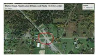
• Station Road, Westmanland Road, Route 161 Intersection. This is a reduced speed limit area (40 mph) for traffic north and southbound on Route 161. Sight distance of southbound traffic on Route 161 is limited due to a sharp dip in the road north of the intersection. Enforcement of the speed limit and installing a flashing traffic signal may reduce the risk of crashes at this area of concern.
