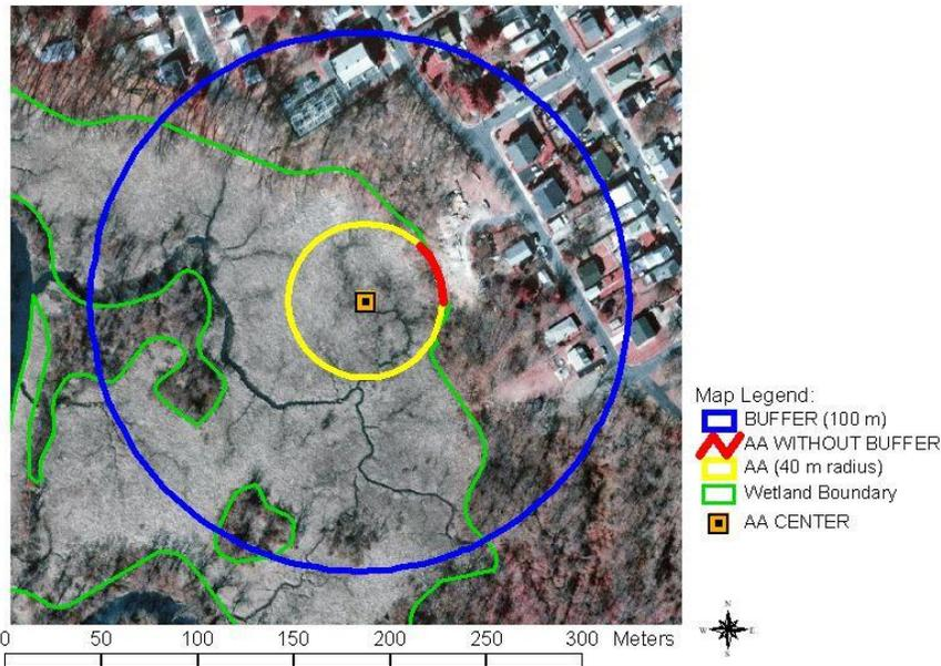
**Example of calculation for Perimeter with Natural Buffer, with simple AA.** The wetland boundary is marked by a thin green line. The assessment area (AA) is shown by the inner circle; yellow indicates portions of the AA perimeter that contain buffer land cover (see “Measurement Protocol” text for definitions) The red indicates that part of AA perimeter lacking a buffer. In this case, about 86% of the AA perimeter has buffer.
