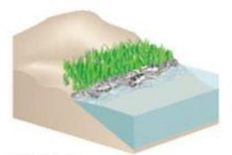
SILLS -Parallel to vegetated shoreline, reduces wave energy, and prevents erosion. Suitable for most areas except high wave energy environments.
