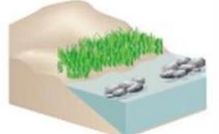
BREAKWATER -(vegetation optional) - Offshore structures intended to break waves, reducing the force of wave action, and encourage sediment accretion. Suitable for most areas.
