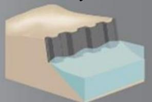
**BULKHEAD** -Vertical wall parallel to the shoreline intended to hold soil in place. Suitable for high energy settings and sites with existing hard shoreline structures.
