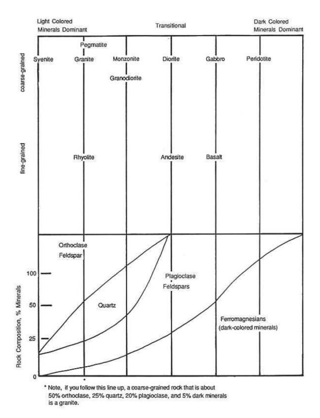
**Figure 2.** Igneous rock identification chart. (Adapted from S. Judson and M. E. Kauffman, 1990, Physical Geology: Prentice-Hall, Inc., Englewood Cliffs, New Hersey, 8th edition.)
