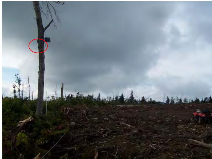
South Stewart Tree Detector: This detector was deployed at this location from August 11 to September 2, 2008 until the met tower was installed. At this location the detector was positioned in a tree approximately 5 m (15') high at the southern edge of the met tower clearing with the microphone facing north into the met tower clearing.
