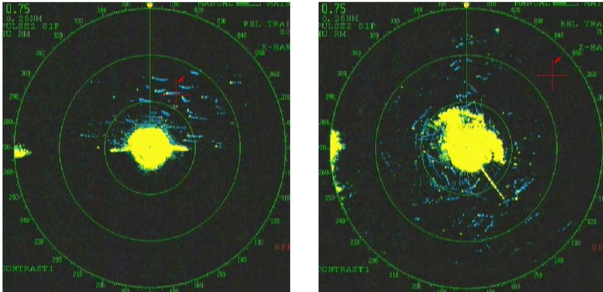
**Figure 2-3.** Radar Screenshot showing ground clutter (yellow). Note the ground clutter is restricted to the center of the radar screen (*left – vertical mode; right – horizontal mode*). Proper site selection can reduce ground clutter to the center of the radar screen, so that the majority of the two-dimensional radar screen remains relatively uncluttered, allowing targets to be tracked as they both enter and leave the cluttered area.
