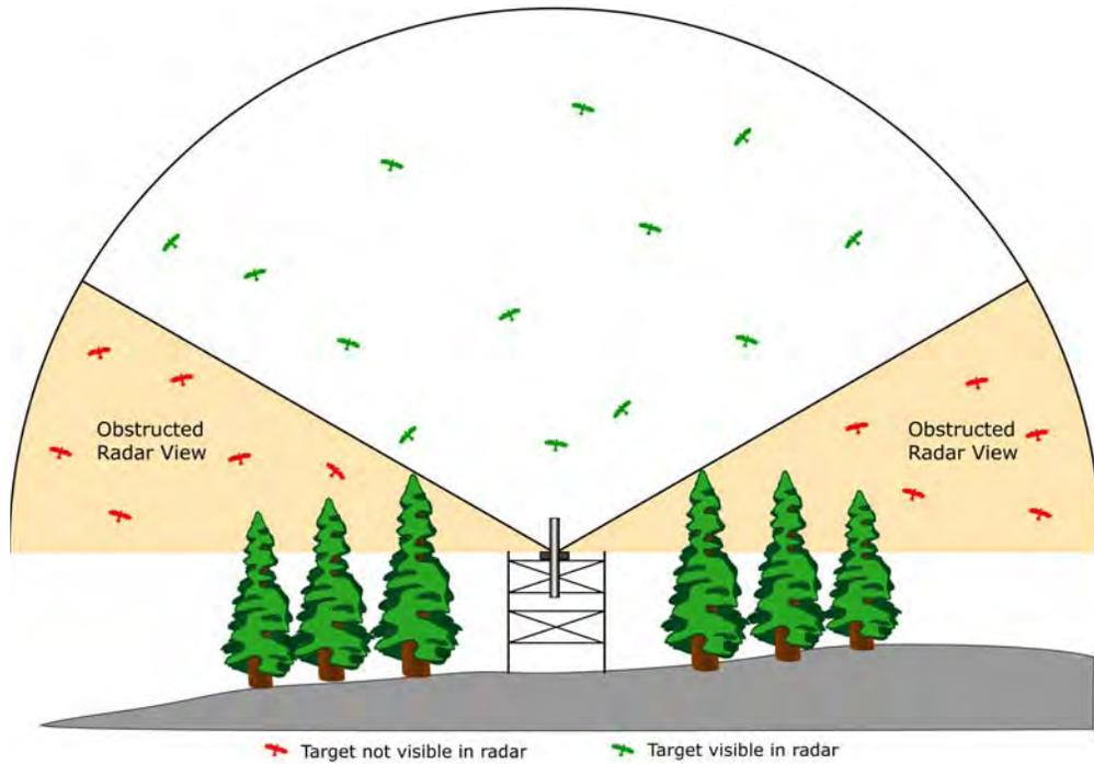
**Figure 2-2.** Examples of surrounding vegetation that causes “ground clutter” obstructions in vertical mode (top) and horizontal mode (bottom). Although the radar records three-dimensional space, it translates ground clutter on the radar screen into a two dimensional representation, which can cause targets to be obscured from view.
