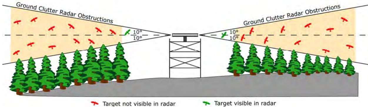
**Figure 2-2.** Ground clutter in horizontal mode (top) and vertical mode (bottom). Although the radar records three-dimensional space, it is translated by the radar screen into a two dimensional representation, which can cause targets to be obscured from view.
