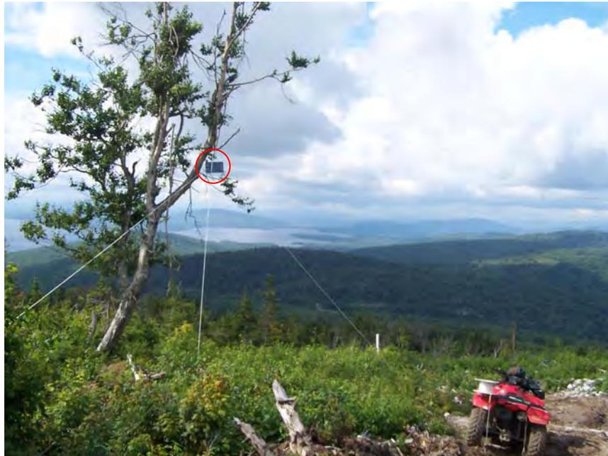
North Stewart Tree Detector: This detector was deployed at this location from August 11 to September 8, 2008. This detector was deployed approximately 5 m (15') up in a tree with the microphone facing east. This detector was located at the northern edge of the met tower clearing where the trail entered the opening on the summit.
