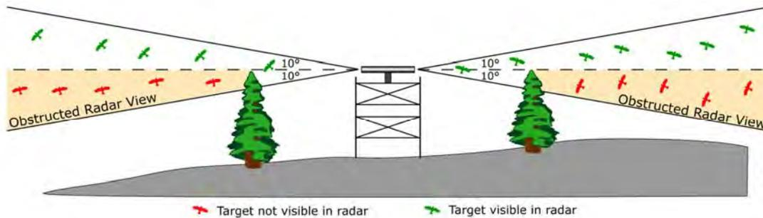
**Figure 2-3.** Proper site selection can reduce ground clutter to the center of the radar screen (top), so that the majority of the two-dimensional radar screen remains relatively uncluttered, allowing targets to be tracked as they both enter and leave the cluttered area (bottom).
