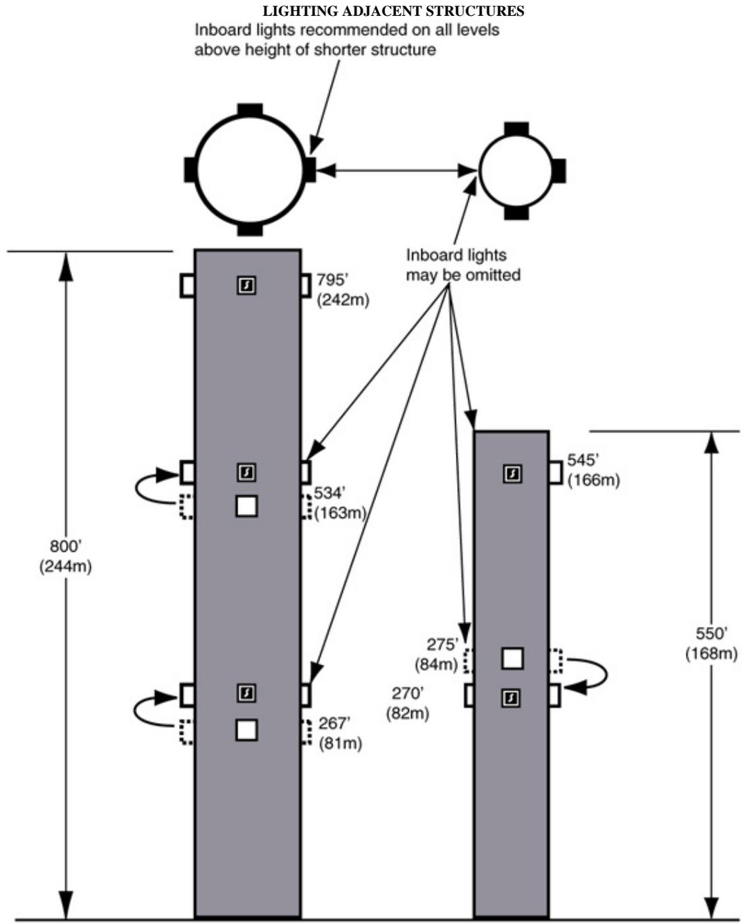
Minor adjustments in vertical placement may be made to place lights on same horizontal plane. Lights on both structures be synchronized
