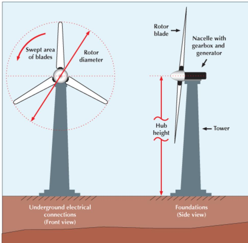
Figure 5. Horizontal Axis Wind Turbine
