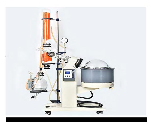
Rotary Evaporator (Roto Vape) – Used in Marijuana Distillate Production
