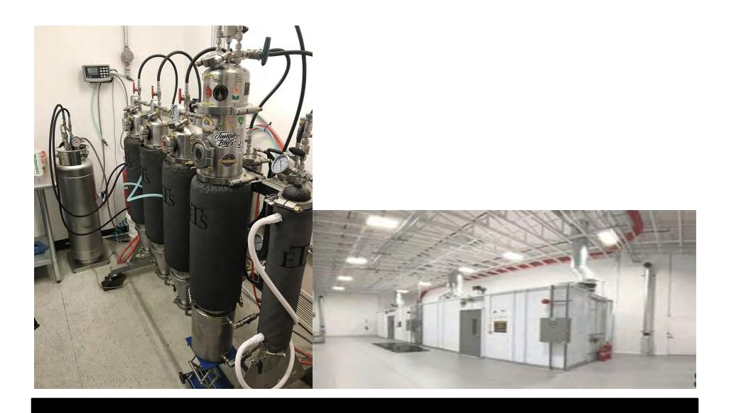
Hydro-Carbon Marijuana Extraction Equipment (Photo 1) and C1/D1 Modular Fire Rated Extraction Booth\* (Photo 2)
