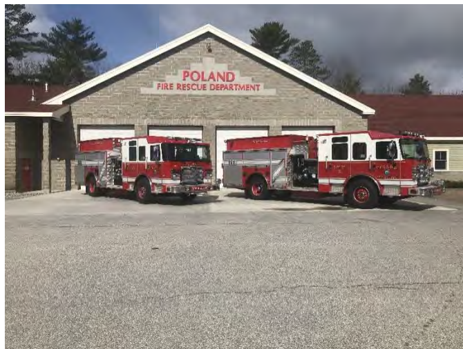
Our fleet of Engines, Engine 2(2016) and Engine 3 (2015) Pierce Enforcers. Each with 1500 GPM pumps, 1000 gallons of water on board.
