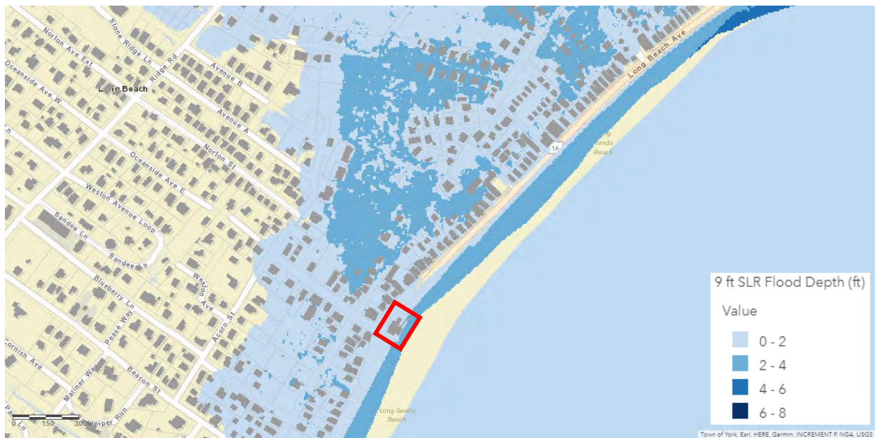
Figure 13. Long Sands Bath House (Red Box) with 9 Feet of SLR and Storm Surge
