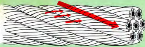
Ordinary right hand lay cable
