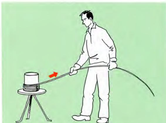
Proper unwinding using a capstan
