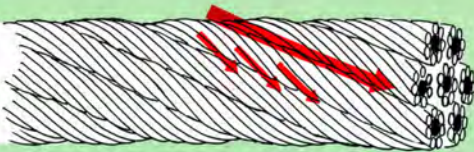
Right hand Lang's lay cable
