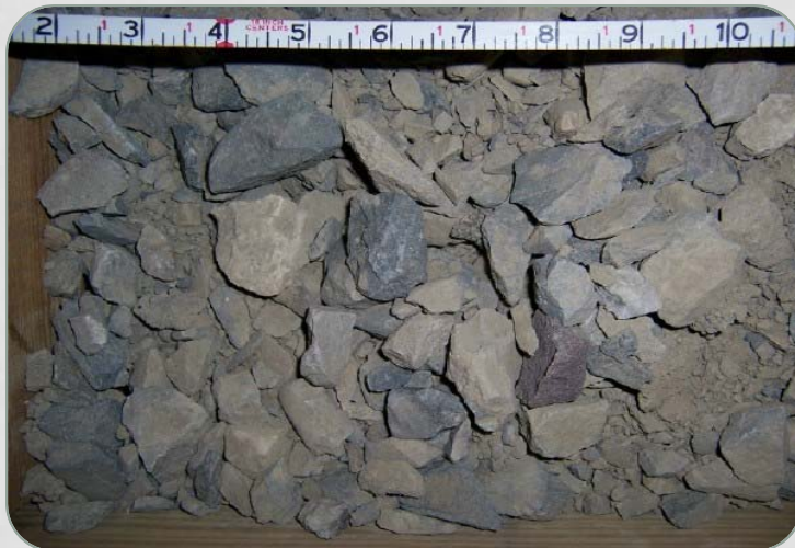
2-inch Crushed Gravel
