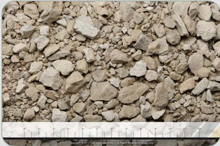
4-inch Crushed Gravel
