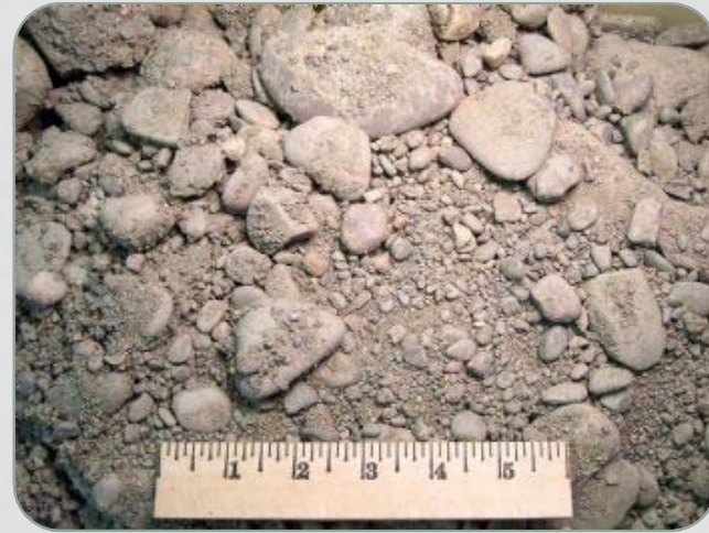
Bank Run Gravel
