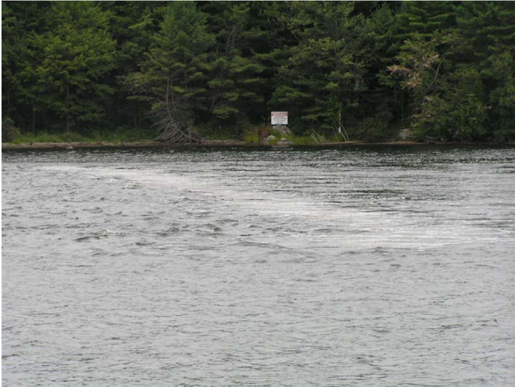
Figure 4: Surface Bubble Pattern of the Existing Oxygen Diffuser at Gulf Island Pond
