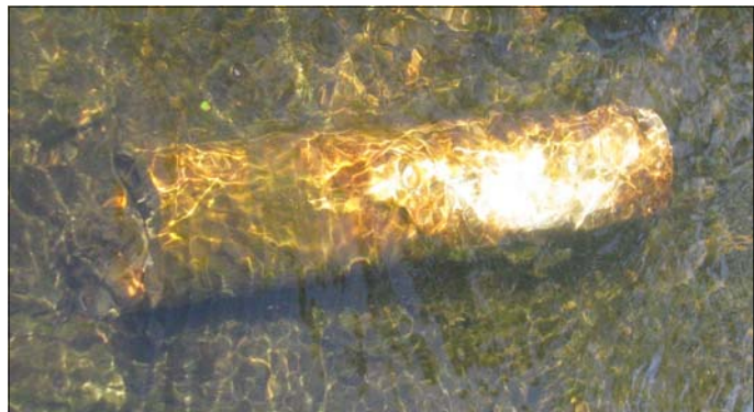
Figure 14. Sonde in PVC protection at Westfield site. Note heavy algae on substrate and PVC.
