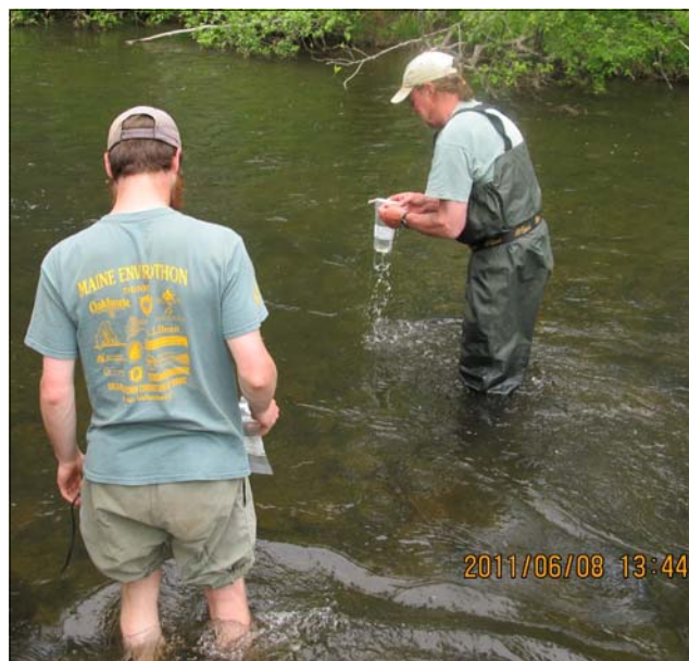
Figure 16. Collecting grab turbidity samples as part of sonde QA.
