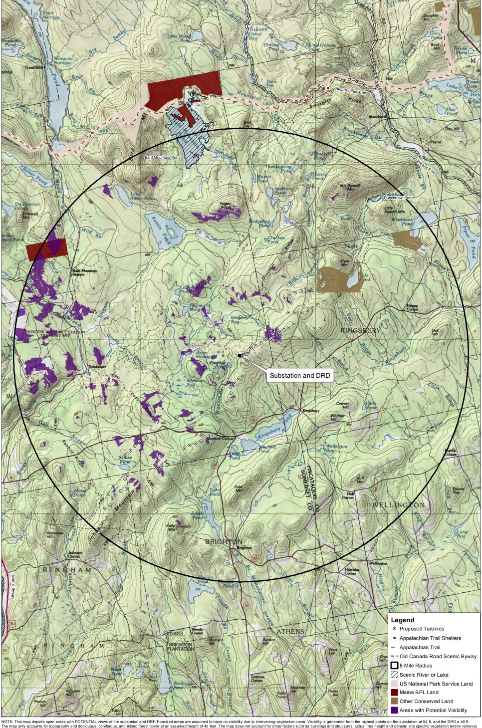
NOTE: This map depicts open areas with POTENTIAL views of the substation and DRF. Forested areas are assumed to have no visibility due to intervening vegetative cover. Visibility is generated from the highest points on the substation at 54 ft, and the DRD a 45 ft.
