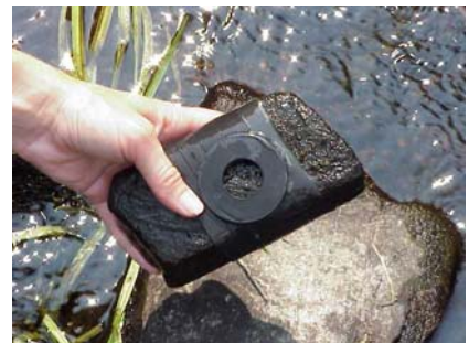
Figure 8: Wrapping sampling device around cobble
