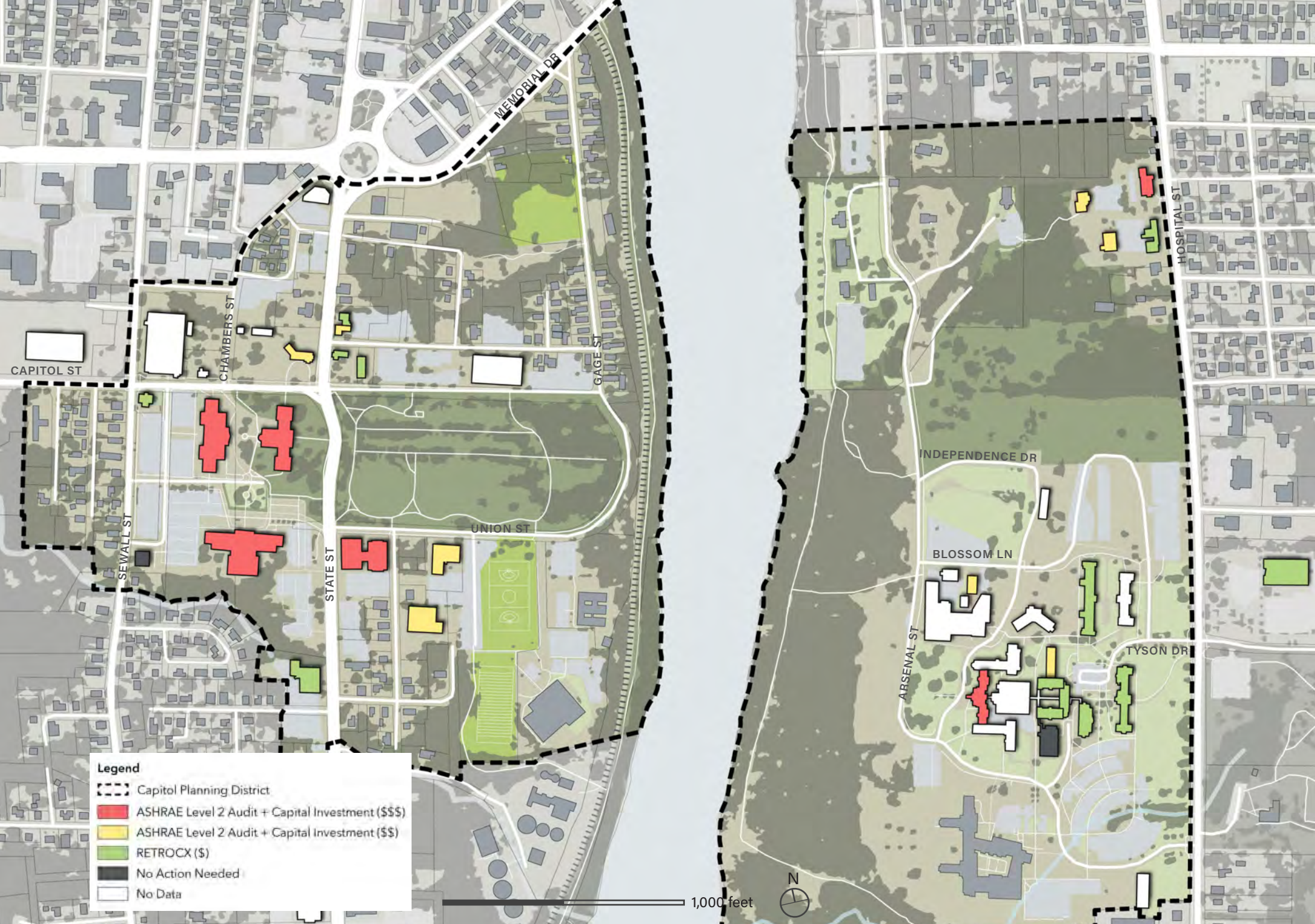
FIGURE 38. FACILITIES ENERGY USE CONDITIONS MAP
