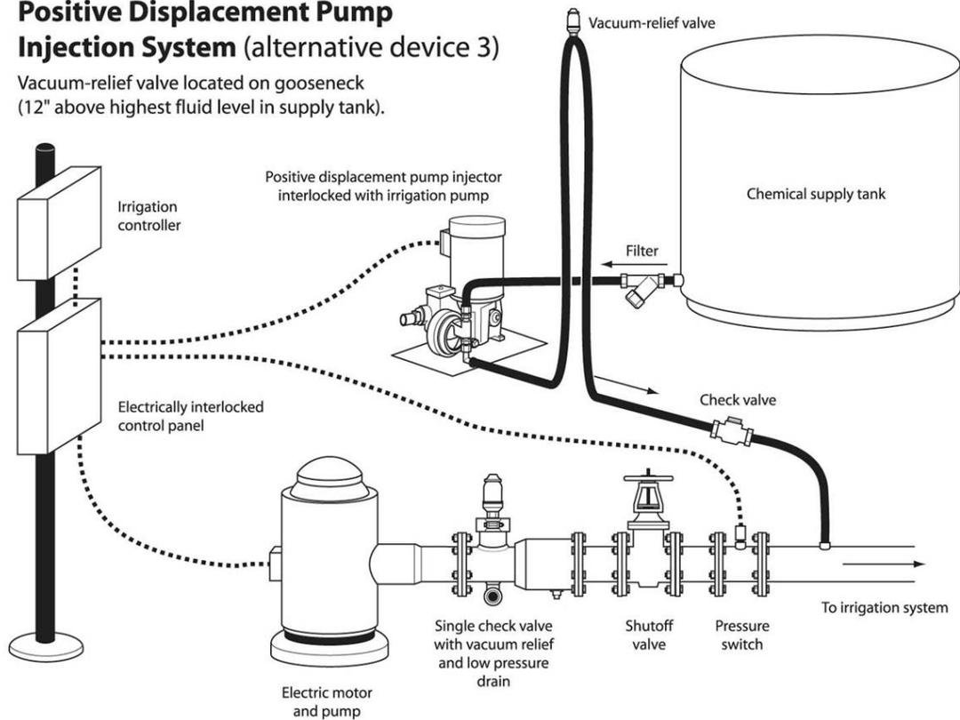
Figure 8: Vacuum relief on pesticide injection pipeline
