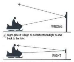
b) Signs placed at the rider's eye level reflect back correctly and are much more visible at night.
