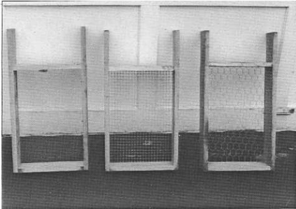
Left to right: 1/4, 1/2, and 1 inch shaker screens for sorting sand/gravel and quarried rock materials. Screens are stacked atop each other in decreasing mesh sizes to sort materials and each screen in turn is gently shaken back and forth. Each screen holds approximately 8-10 pounds of material.
