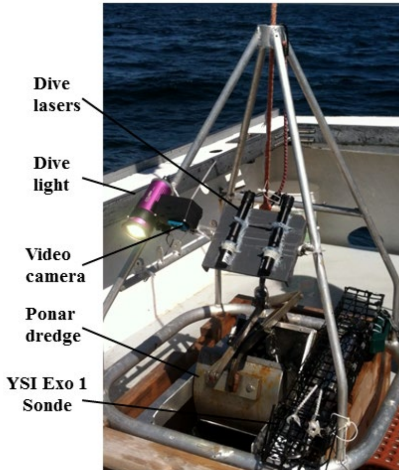
Figure 3. MCM grab sampling platform.
