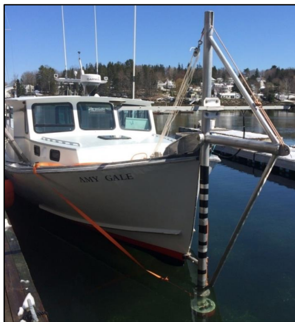
Figure 4 – F/V Amy Gale shown with pole-mounted dual GPS antennas, Kongsberg EM2040C multibeam sonar, MRU (not visible), and surface sound speed probe (not visible) in acquisition mode
