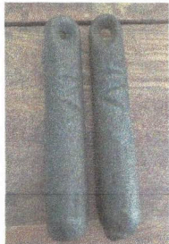
Counter weight - for depth control line ~10 lbs
