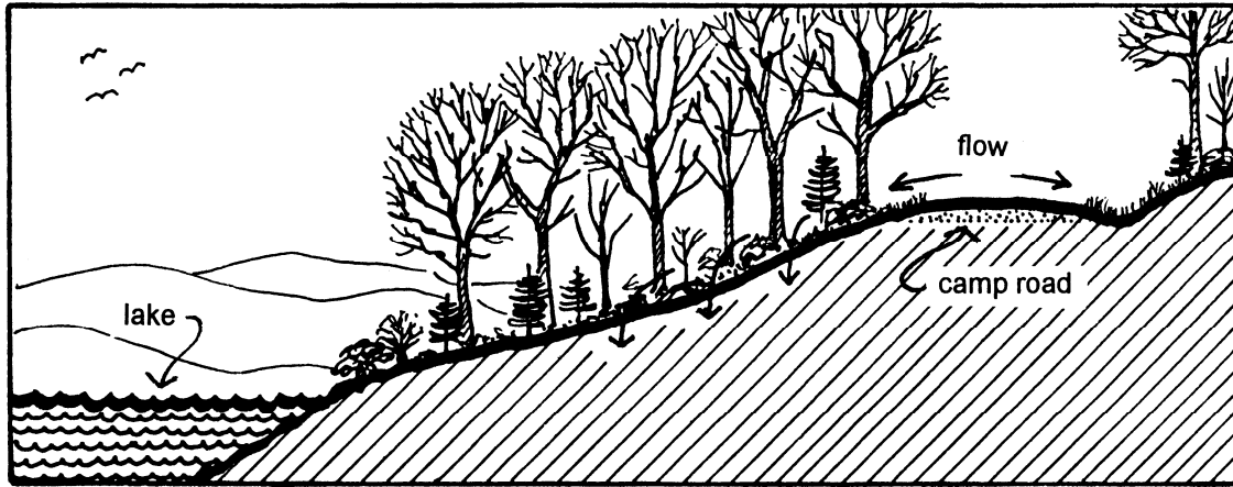
Figure 4. Vegetated buffers filter and absorb camp road runoff.
