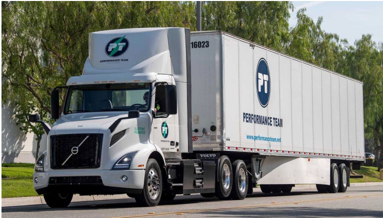
Figure 5.2 Volvo VNR battery powered truck presently has a range of up to 275 miles
